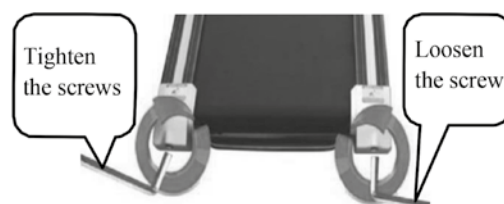
Figure A Adjustment method of running belt biased to the left
